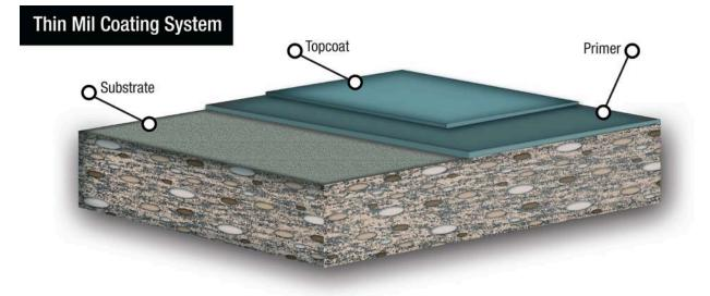
Thin Film Industrial Floor is a colored epoxy/urethane, high performance concrete coating system. It is used for environments requiring an attractive, economical, high performance floor.
